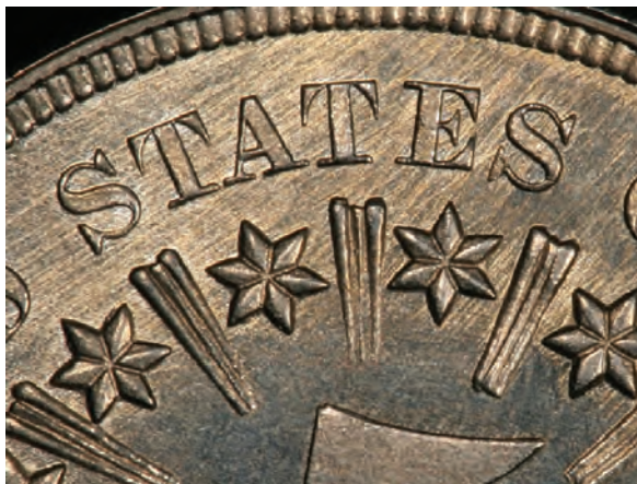
Lapping on the Reverse Used to Strike 1867 With Rays Proofs State e, the loss of detail of the rays under the first S of STATES is not seen in State d
