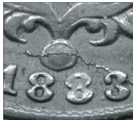
▲ 1883/2 FS-013.1: Underlying 2 clearly visible slightly to left of 3; die break from rim through 3 and ball.
